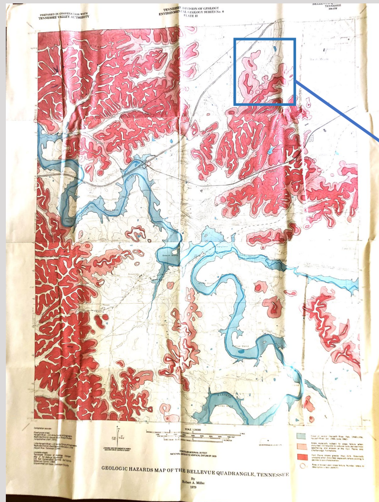
Fig. 3. Bellevue Quad: Harpeth River flowing from SE to NW. Slope failure hazards in pink and red.
