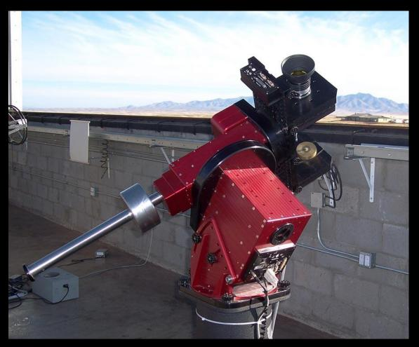
Located in South Africa Consists of Paramount ME Apogee Alta U16 CCD Camera Mamiya 80mm f/1.9 Lens with 42mm aperture
