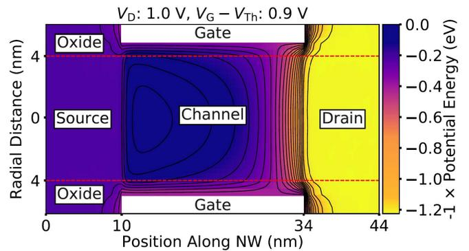
Fig. 3. Electron potential energy along the x-direction of the cylinder in Fig. 1(c), illustrated with a color map. The density of the equipotential lines reflects the magnitude of the electric field. Metallurgical junction boundaries are at  $x = 10$  and  $34$  nm. The red dashed lines separate the oxide and semiconductor regions of the device. The aspect ratio is different from actual device dimensions for clarity.
