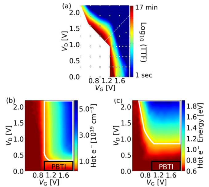
Fig. 7. (a) Experimentally derived time-to-failure (TTF) maps of the GAA device, adapted from Chasin *et al.* [7]. (b) Simulated density of hot carriers in a small volume near metallurgical junction  $\sim$  within  $\pm 2$  nm in the x-direction. (c) Simulated average KE of these hot electrons. Only the electrons with energy higher than 0.5 eV are considered for subplots (b) and (c). Scales of the color bars in (a) are logarithmic, and those in (b) and (c) are linear.
