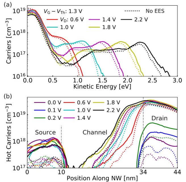
**Fig. 5.** Energy distribution of electrons for several drain biases at  $V_{GS} - V_{Th} = 1.3 \text{ V}$ . (a) Electron-energy histogram within 2 nm in each direction of the metallurgical drain junction. (b) Density of electrons above 0.5 eV in the NW. The dotted curves show results without including EES.
