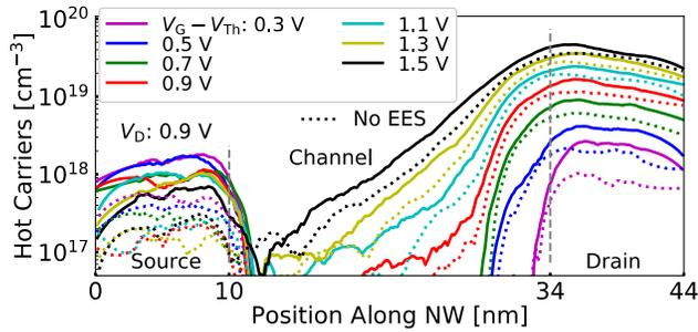
Fig. 6. Density of electrons above 0.5 eV in the NW for several overdrive biases at  $V_{DS} = 0.9$  V. Dashed lines show the hot-electron distribution without EES.
