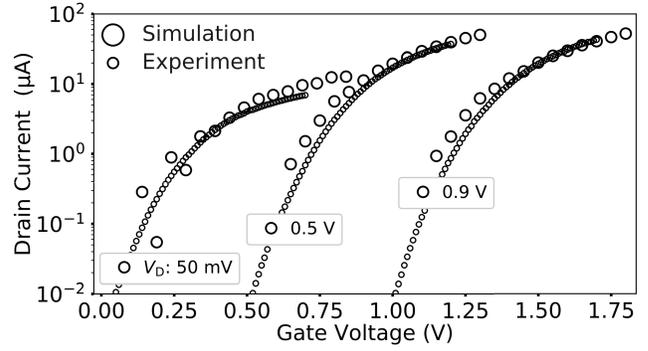
Fig. 2. Experimental and simulated gate control at 50-mV, 0.5-V, and 0.9-V drain bias. Curves are shifted along the x-axis by  $-0.5$ ,  $0.0$ , and  $0.5$  V, respectively. The experimental drain current is divided by 2 to match the simulated  $I$ - $V$  characteristics of the single NW structure depicted schematically in Fig. 1(c).
