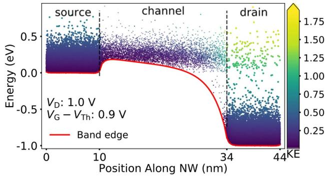
**Fig. 4.** Carrier KE distribution above the conduction-band edge along the  $x$ -direction of the device. The conduction-band edge is averaged over the cross section of the channel. Statistical carrier enhancement within the dashed vertical lines ensures adequate sampling of interactions in an otherwise sparsely populated region. The KE of the carriers is represented by both particle color and the distance above the conduction band.
