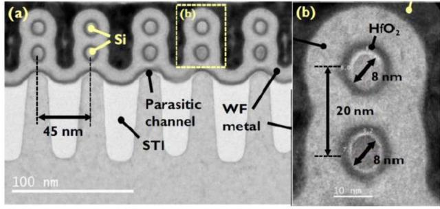
Fig. 1. TEM images of a GAA Si nMOSFET from imec [53] depicting (a) NW array and (b) single NW vertical stack. WF metal represents the work-function metal used for the gate electrode. (c) Schematic of the simplified device used for simulation (not drawn to scale). The insulating oxide in the S/D access region and gate contact extends radially outward until the end of the tensor mesh (not shown).
