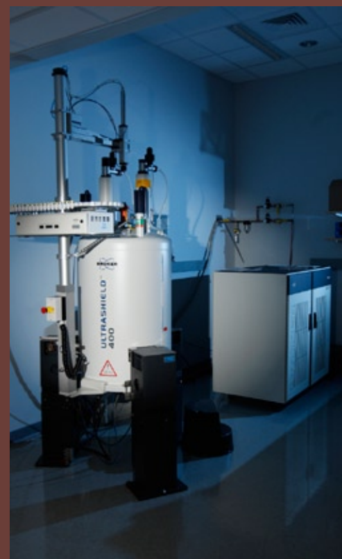
400 MHz FT-NMR DRX spectrometer with sample changer (BACS 60)
