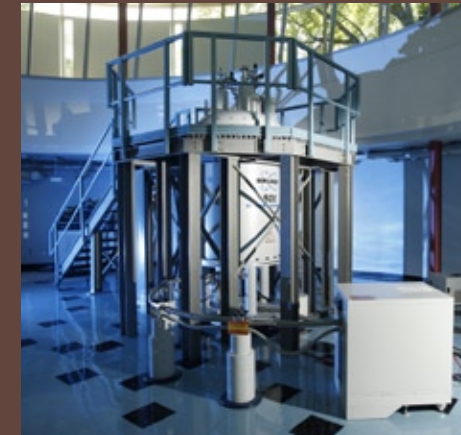
800 MHz Bruker Avance FT-NMR spectrometer with cryoprobe
